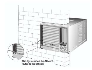
• Place the front grille on the cabinet first. Secure the front grille to the main chassis using screw provided.
